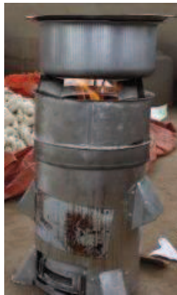
FIGURE 9 - Top Lit Updraft stove (MWOTO stove – Uganda)
